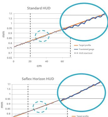
Compared with standard HUD interlayers, the improved sheet thickness uniformity provided by Saflex Horizon LVID HUD creates a wedge angle that remains closer to target throughout the HUD zone, resulting in a reduction in localized image ghosting. In addition, the reduction in the wedge angle rate of change further improves driver experience by reducing dynamic ghosting.
